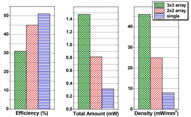
Fig. 10. Simulation results: power transfer efficiency, total delivered amount, and power transfer density of three cases
