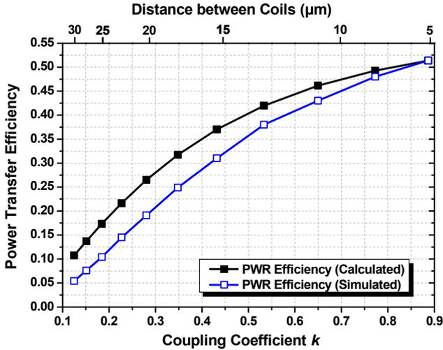
Fig. 7. Coupling coefficient  $k$  vs. power transfer efficiency
