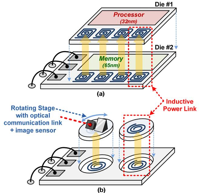
Fig. 1. The applications of wireless power transfer using inductive coupling: (a) Vertical stacking of heterogeneous processes such as logic and DRAM (b) Information Tethered Micro Automated Rotary Stages (ITMARS). Sensors and communication link are integrated on a rotating stage in a substrate.
