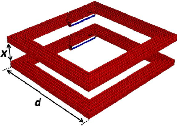
Fig. 6. Two vertically stacked coils for wireless inductive power link
