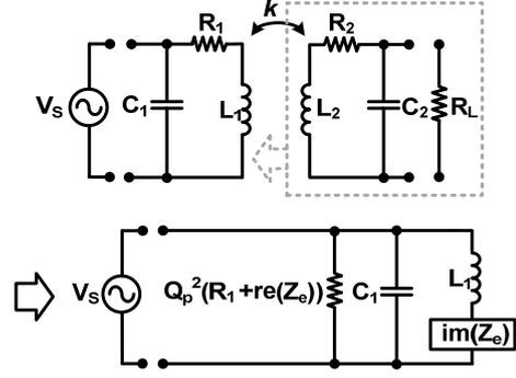
Fig. 5. Equivalent circuit for power density calculation
