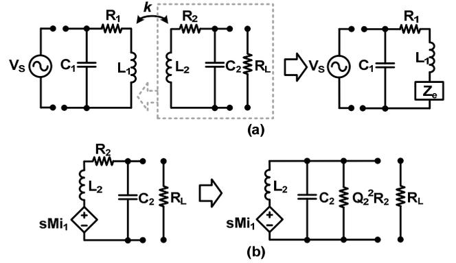
Fig. 3. (a) Entire equivalent circuit (b) Secondary equivalent circuit
