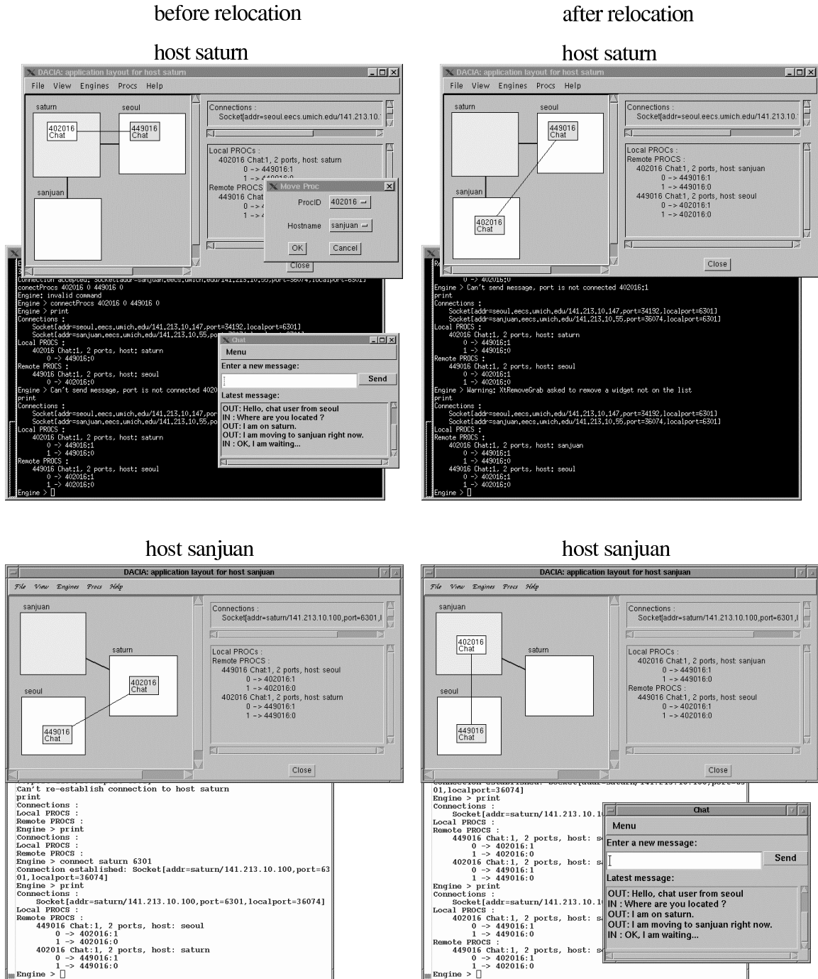
Figure 4.10: A Chat PROC moves from one host (saturn, top left) to another one (sanjuan, bottom right). All PROCs remain connected and continue to exchange data. The graphical interface windows on each host show the configuration of the application, both for the local and remote hosts. Squares represent hosts, and small labeled rectangles represent PROCs. The graphical interface in the top left corner shows two connected Chat PROCs, one situated on the local host (saturn) and one on the remote host (seoul). The terminal windows show application status information, as displayed by the command-line interface.
