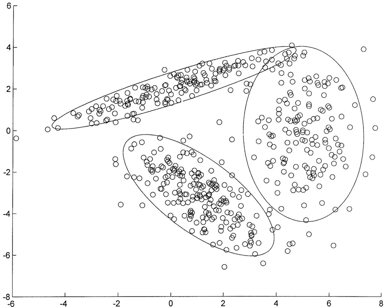
In these notes we'll develop a general method for clustering data when clusters are elliptical, based on maximum likelihood estimation of GMMs.
