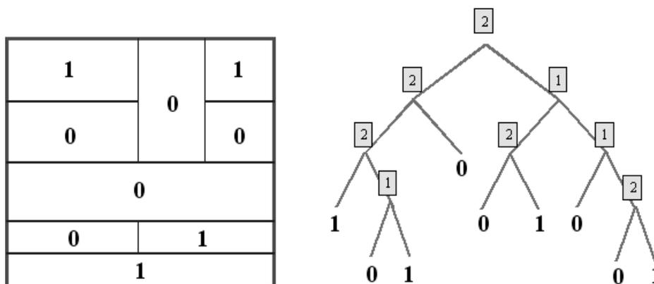
Figure 2: A dyadic decision tree (right) with the associated recursive dyadic partition (left) in  $d = 2$  dimensions. Each internal node of the tree is labeled with an integer from 1 to  $d$  indicating the coordinate being split at that node. The leaf nodes are decorated with class labels.
