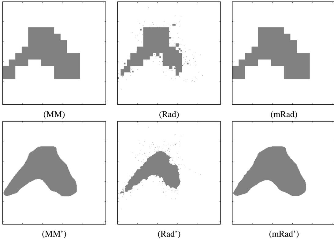
Figure 9: Minimum volume set estimates based on dyadic quadrees for  $\alpha = 0.90$  with  $n = 1000$  samples. Reconstructions based on MM = minimax penalty (23), Rad = Rademacher penalty (24), and mRad = modified Rademacher penalty (25), and MM', Rad', and mRad' denote the analogous estimates based on voting over multiple trees at different shifts.
