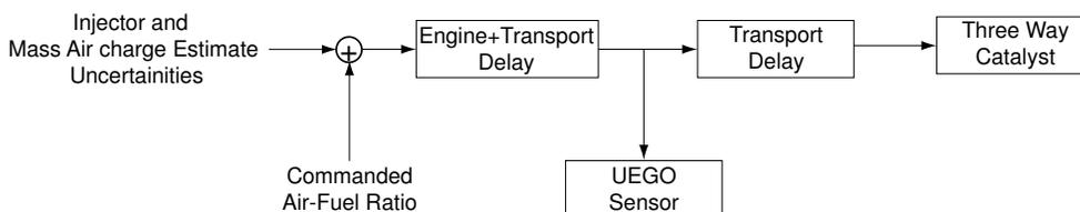
Fig. 2. Simplified engine model.
