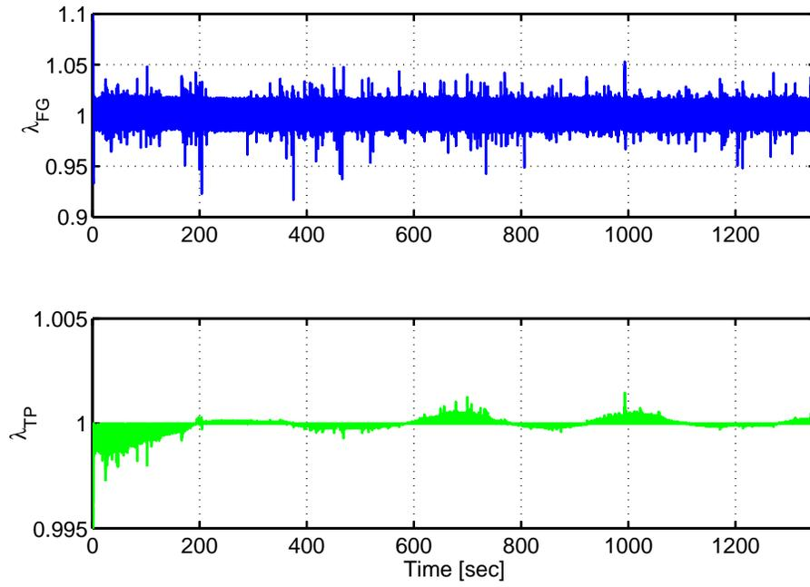
Fig. 9. Air-Fuel ratio at feedgas and tailpipe.
