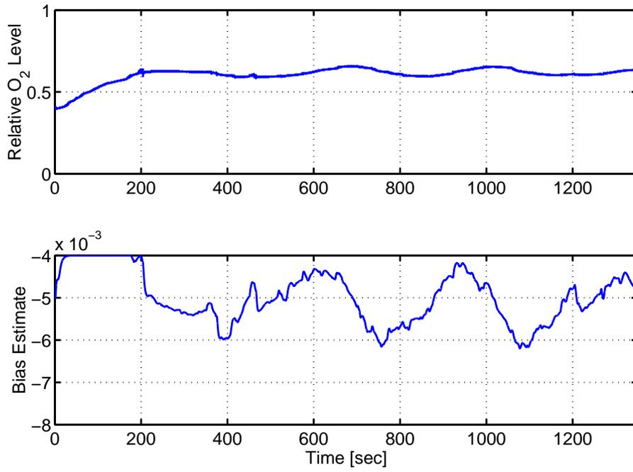
Fig. 11. Relative oxygen level and estimated bias.
