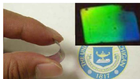
FIG. 3. (Color online) Photograph of a flexible conjugated polymer solar cell with controlled nanoscale heterojunctions. Inset: TDPTD on a flexible ITO-coated PET, imprinted with a 700 nm period grating mold, diffracting ambient light.
