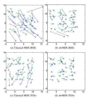
**Fig. 3.** Experimental sensor network location estimates from RSS and TOA measurements via MDS method and dwMDS method (using adaptive neighborhood selection w/  $d_R = 6$  m). Anchor nodes 'x', true sensor locations 'o' and location estimates 'v' are shown.
