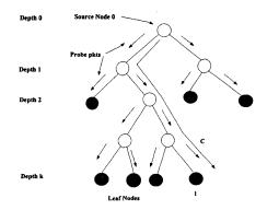
Fig. 1. Multicast Distribution Tree. All nodes in tree participate in a session during which cummulative multicast link losses are reported to all participants, e.g via RTCP. The solid circles denote edge nodes to which multicast packets are sent from the source node. The path C denotes the particular chain investigated by the ML algorithm using loss statistics along chain C only.
