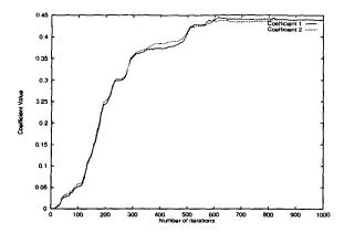
Figure 1: Trajectory of  $w_{1,k}$  and  $w_{2,k}$  for  $\mu = 0.005$
