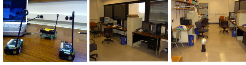
Figure 3.4: Experimental platform: wireless Mica2 sensor nodes.
