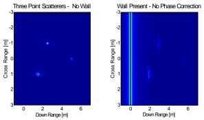
Figure 2.2: Point Simulation – (left) No Wall (right) Wall Inserted
