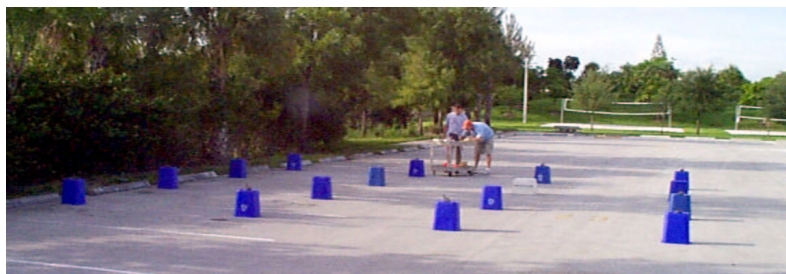
Fig. 8. Parking lot testbed experiment. Devices are located on top of 16 upside-down recycling bins.
