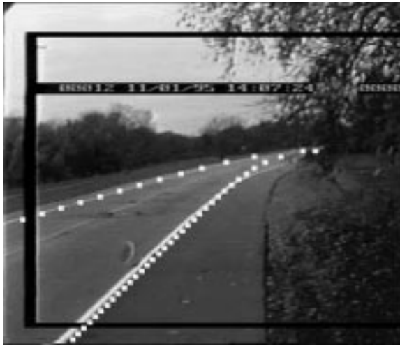
(a) Single sensor based lane edge detection
