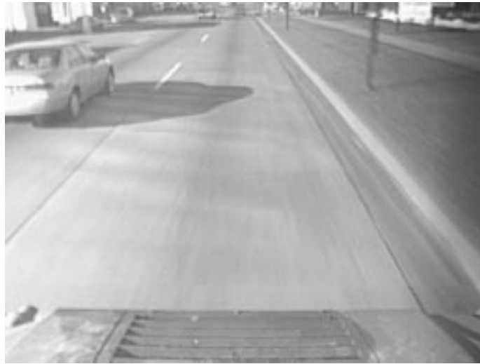
Figure 5.1.1: Clutter due to presence of complex shadows
