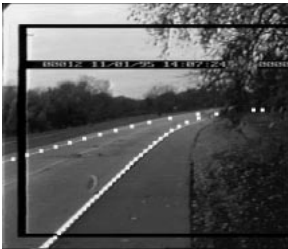
(c) Lane edge detection with fusion method
