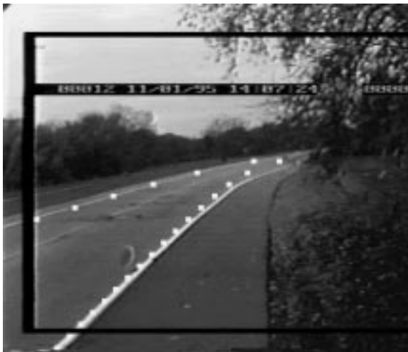
(c) Lane edge detection with fusion method
