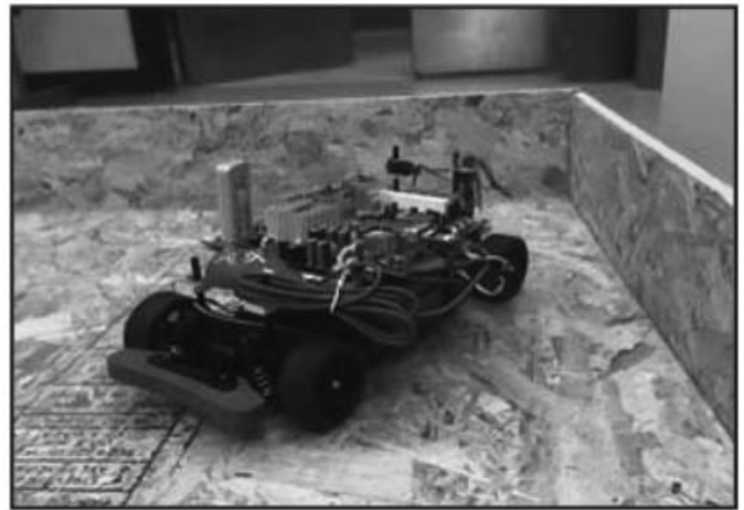
Fig. 6. Experimental vehicle employing hardware-in-the-loop simulation.
