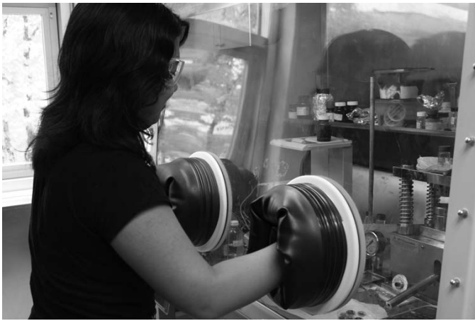
Fig. 1. A camper putting together a button Li-Ion battery.
