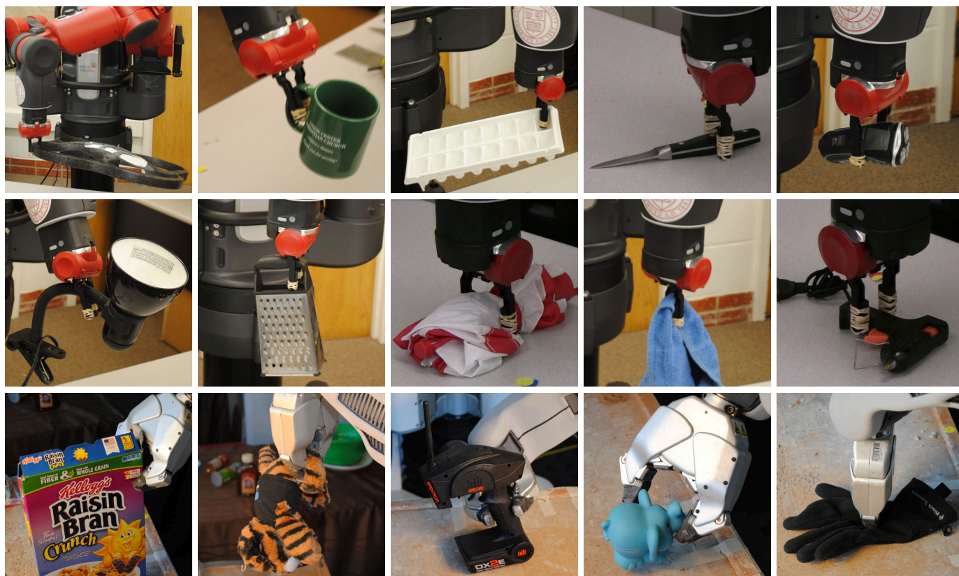
Fig. 15: Robots executing grasps: Our robots grasping several objects from the experimental dataset. Top row: Baxter grasping a quad-rotor casing, coffee mug, ice cube tray, knife, and electric shaver. Middle row: Baxter grasping a desk lamp, cheese grater, umbrella, cloth towel, and hot glue gun. Bottom row: PR2 grasping a plush cat, RC car controller, cereal box, toy elephant, and glove.
