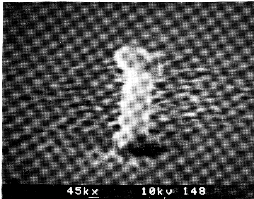
Figure 4. An SEM micrograph of a 0.3\ \mu\text{m} \times 0.3\ \mu\text{m} Nb junction area for which a successful \text{SiO}_2 based trilevel resist feature was obtained. The shrinkage from the mask feature size of 0.8\ \mu\text{m} \times 0.8\ \mu\text{m} is primarily due to the "undercutting" of the Nb film in the high pressure \text{CF}_4 + \text{O}_2 etch. A lateral shrinkage of 0.25\ \mu\text{m} < x_{\text{shrink}} < 0.35\ \mu\text{m} was therefore required for this successful polyimide shrink step. This step is performed, however, without quantitative information on the extent of the Nb undercutting, resulting in poor repeatability.
