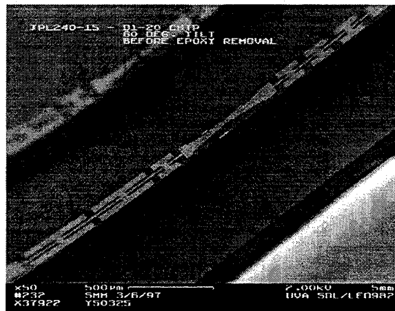
Figure 6: Complete 240 GHz mixer
