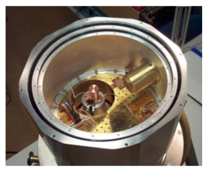
Fig. 5 The current phase in installation of the new system. One can see the <sup>3</sup>He-cryocooler mounted in a pit in the 2 K-cold plate of an 8-inch HDL dewar from Infrared Labs and a long baffle (here blanked), which will accommodate the stimulator and the filter unit. This longer baffle is exchangeable with a shorter one for the filter unit only.
