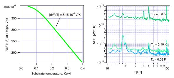
Fig. 2 Experimental results: left panel – calibration curve for the NIS junction thermometer, no heating is applied to the sensor; right panel – electrical Noise Equivalent Power of the sensor measured at three different substrate temperatures.
