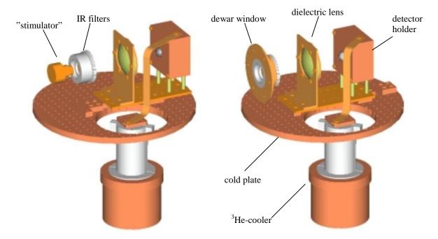
Fig. 6 Computer-generated images of the components inside the <sup>4</sup>He dewar. Left side – option for measurements with an internal stimulator; right side – option for measurements with irradiation through the dewar window. The two configurations can be exchanged by simple re-mounting of the filter unit and shifting the smaller optical bench along the optical axis.
