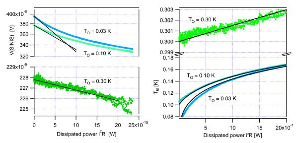
Fig. 3 Experimental results: left panel – electrical responsivity of the power sensor (voltage at the output of the thermometer vs. heating applied to the absorber) for three substrate temperatures  $T_0$ ; black lines show the small-signal responsivity.
