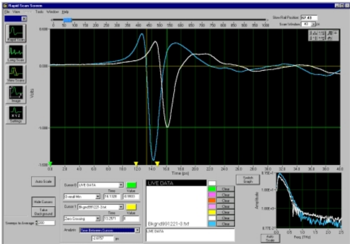
Figure 5. Rapid-scan acquisition screen for the time-domain terahertz spectrometer software. The main graph shows two time-domain traces. The white trace is the live, rapidly updated THz scan which has passed through a latex balloon. The gray trace is a saved background scan. The secondary graph shows the Fourier transforms of the two traces.
