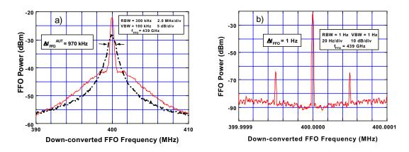
**Fig. 3.** [7] The down-converted IF power spectra of the FFO (f = 439 GHz), recorded with different frequency spans, clearly demonstrate the phase locking.
