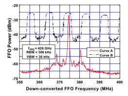
**Fig. 5**. Down-converted FFO signal recorded at constant bias current adjusted inside one of the resonances (curve A) and in between two resonances (curve B).
