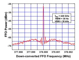
**Fig. 9.** Down-converted spectra of the FFO operated at 426 GHz; frequency locked (curve A) and phase locked (curve B).
