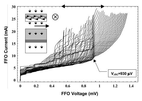
Fig. 1. IVCs of a Nb-AlO<sub>x</sub>-Nb FFO recorded at different magnetic fields. Note the abrupt change of the IVC at the boundary voltage  $V_{JSC} \approx 930 \,\mu\text{V}$ . Insets show the cross section of the long junction with driven vortices (top) and its overlap geometry (bottom).
