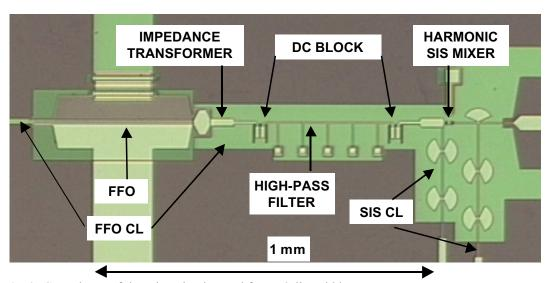
Fig. 2. Central part of the microcircuits used for FFO linewidth measurements.
