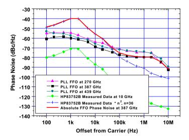
**Fig. 4.** Experimental phase noise of a phase locked FFO at different frequencies. Since the phase noise of the FFO, e.g., at 387 GHz is measured relative to the  $36^{th}$  harmonic of the synthesizer, the synthesizer noise, multiplied by a factor  $36^2 = 1296$ , should be added to residual FFO noise to get the total (absolute) FFO phase noise – solid line.
