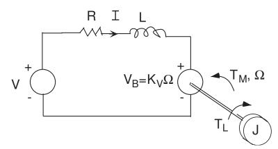
Input: applied voltage, Output: current, torque, speed
