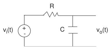
Input: applied voltage, Output: voltage across capacitor
