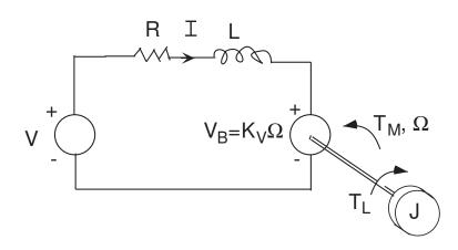
• Suppose motor is driven by a constant voltage source. Then steady state speed and torque satisfy
