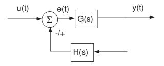
• *Feedback equations*: the output depends on the error, which in turn depends upon the output!
