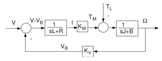
Transfer function from Voltage to Speed (set T<sub>L</sub> = 0):
