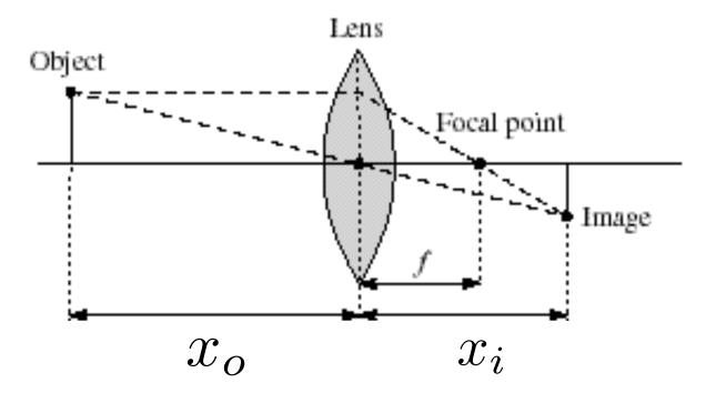
How to relate distance of object from optical center (x<sub>o</sub>) to the distance at which it will be in focus (x<sub>i</sub>), given focal length f?
