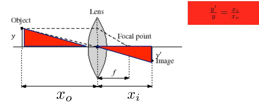
How to relate distance of object from optical center (x<sub>o</sub>) to the distance at which it will be in focus (x<sub>i</sub>), given focal length f?
