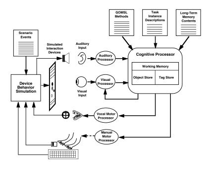
Figure 1. Architecture of the GLEAN system.
