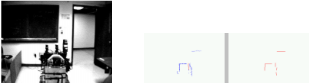
Figure 9.5: The robot is facing a door from inside a room toward a corridor. On the right a two dimensional plot of the laser scan with an extra line indicating the bisector of the doorway recognized by the robot. The rightmost figure shows the segments used to detect the doorway. A doorway is recognized by finding two perpendicular segments with open space between them.
