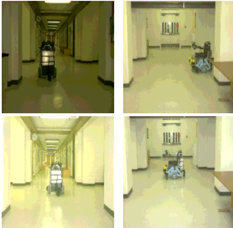
Figure 9.7: Hill climbing to a corridor intersection. The top row illustrates two views of the initial robot location before hill climbing. The bottom row illustrates the corresponding views after hill climbing.
