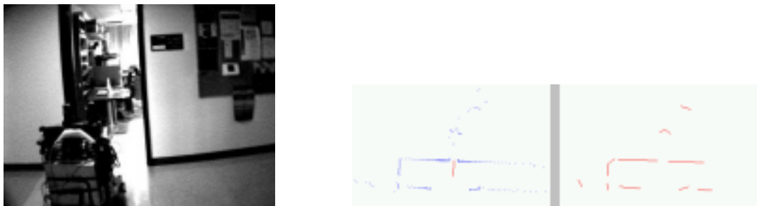
Figure 9.6: The robot is looking inside a room from a corridor. On the right a two dimensional plot of the laser scan with an extra line indicating the bisector of the doorway recognized by the robot. The rightmost figure shows the segments used to detect the doorway. A doorway is recognized by finding two collinear segments with open space between them.
