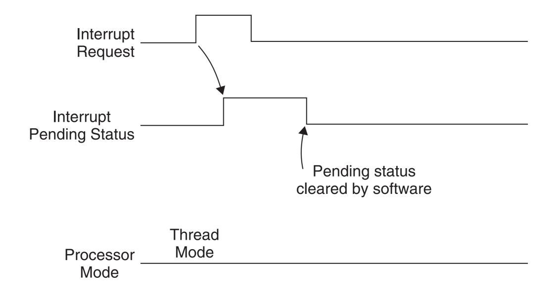
Software clears pending status while PRIMASK/ FAULTMASK is 1
