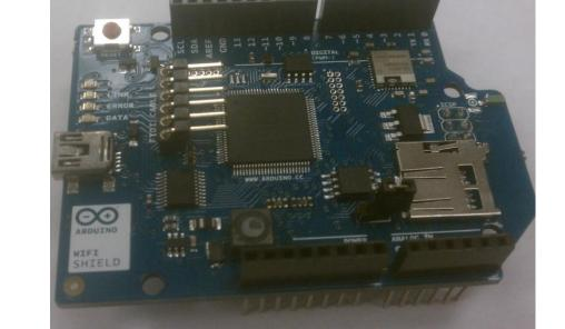
The WiFi module functions as a server mounted on the machine. The Apache server then runs a script to act as a client and connect to the WiFi module. The information for the current drink order is then embedded in the URL that the Apache server uses to access the WiFi module.
