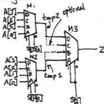
Also, note that there are other possible designs. For example, if mux M3's S<sub>1</sub> and S<sub>0</sub> inputs are connected to φ and S[2], respectively, then M3.A = tmp1 and M3.B = tmp2, rather than the way it is drawn here.
