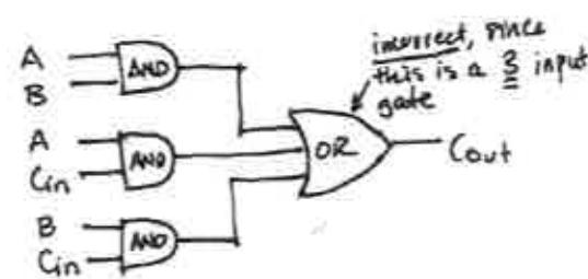
↓ redrawn using 2 input gates
