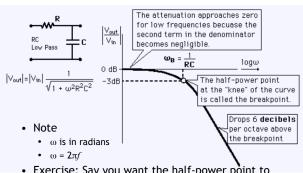
Exercise: Say you want the half-power point to be at 30Hz and you have a 0.1 µF capacitor. How big of a resistor should you use?
