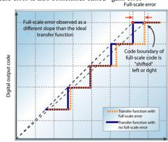
full-scale error is the difference between the ideal code transition to the highest output code and the actual transition to the output code when the offset error is zero.
