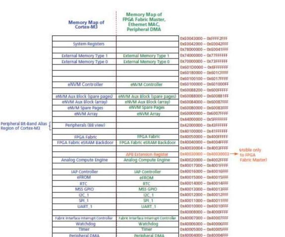
UART 0 0x40000000 - 0x40000FFF UART\_0 0x24000000 - 0x3FFFFFFF SRAM Bit-Band Alias eSRAM\_0 / eSRAM\_1 (BB view) 0x22000000 - 0x23FFFFFF Region of Cortex-M3 0x20010000 - 0x21FFFFFF eSRAM 1 eSRAM 1 0x20008000 - 0x2000FFFF Cortex-M3 System Region eSRAM\_0 eSRAM 0 0x20000000 - 0x20007FFF ....... 0x00088200 - 0x1FFFFFFF Cortex-M3 0x000881FF Code Region
