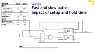
Assume that the input A is coming from a flip-flop that has the same properties as the flip-flops that are shown and is clocked by the same clock
