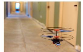
Figure 1: One SensorFly node hovering in the hallway.
