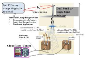
Figure 2: Ultra low cost pervasive computing Grid convergence architecture. The wireless computational processing, cell site processing, Net-PC processing, and remote application en services are all displaced via wireless and (radio) fiber optics from there local site to the cloud data center.
