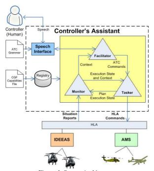
Figure 1. System Architecture.
