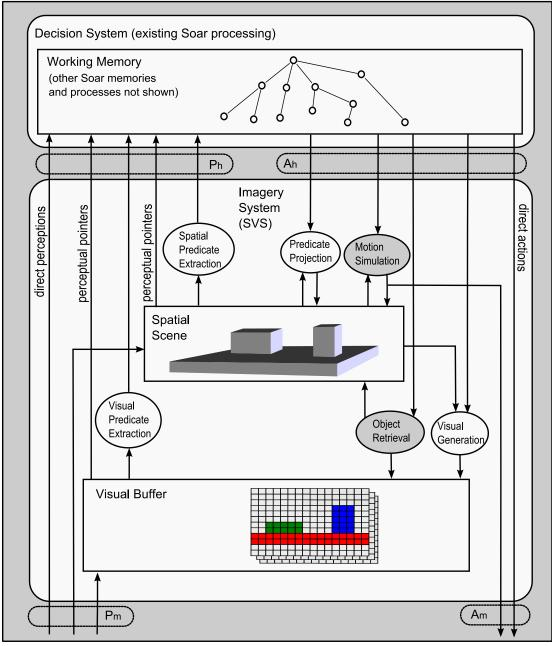
Figure 2: SVS System design. Boxes are short-term memories, circles are processes. Grey circles involve access to information in long-term memory (knowledge). There are implicit control lines (not shown as arrows) between working memory and all of the processes shown.
