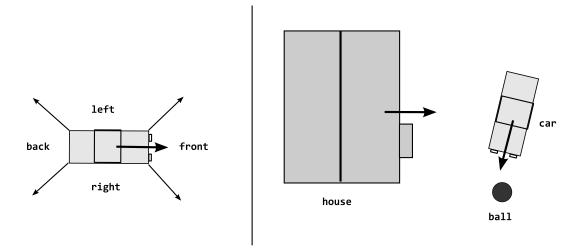
Figure 7: Orientation information in SVS (two-dimensional simplification). Left: The intrinsic front vector of the car object, along with its shape, defines four acceptance areas, which are used to define qualitative orientation information. For example, an object in the region labeled "right" is considered to be to the right of the car.
