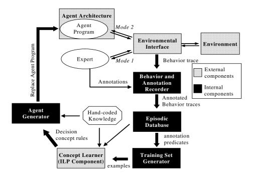
**Fig. 1.** General overview of our learning by observation framework. In mode 1, the expert generates annotated behavior. In mode 2, an agent program executes behavior and the expert accepts or rejects its annotations
