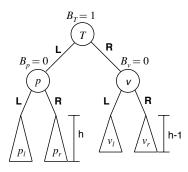
AVL balanced at T, p, and v
