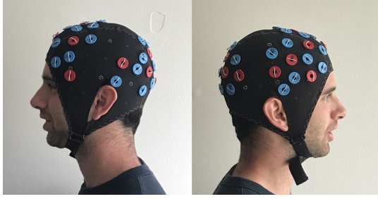
Fig. 1: fNIRS cap used in our experiments. Red circles are light transmitters while blue circles are light receivers. fNIRS is only able to observe brain activation on channels between nearby transmitters and receivers.
