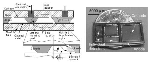
The microGeiger can detect and distinguish the energy of incident beta particles, allowing identification of lethal radioisotopes.
