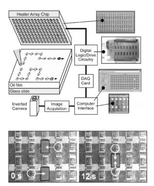
Schematic of the programmable system for noncontact droplet actuation based on Marangoni flows. The system includes a 128pixel array of resistive heaters suspended above the oil layer, control circuitry, and a graphical user interface.
