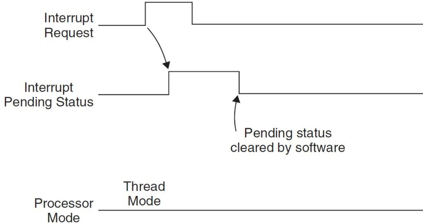
In this case, the processor never took the interrupt because we cleared the IPS by hand (via a memory-mapped I/O register)
