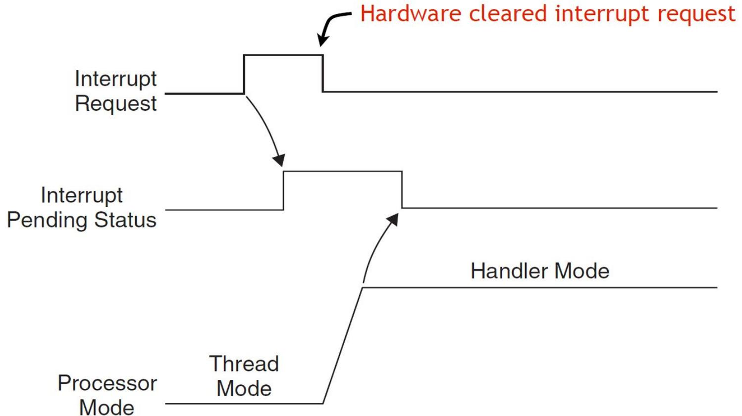
The normal case. Once Interrupt request is seen, processor puts it in “pending” state even if hardware drops the request. IPS is cleared by the hardware once we jump to the ISR.
