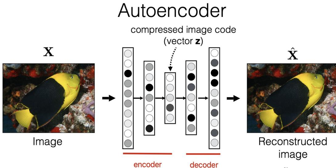
vector  $z$ (output of encoder) is also the representation of the original image
