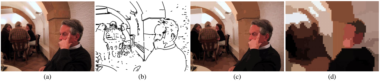
Figure 2: (a) Original image; (b) Detected edges; (c) Color segmentation; contiguous regions of solid color in these images represent individual elements of the segmentation; (d) Color segmentation at a coarser scale (the image was first down-sampled by a factor of 16)
