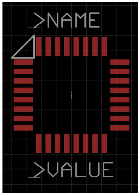
Using the 'wire' command place a pin 1 mark on layer '21 tPlace' like in the picture. This will be used when assembling the board.
