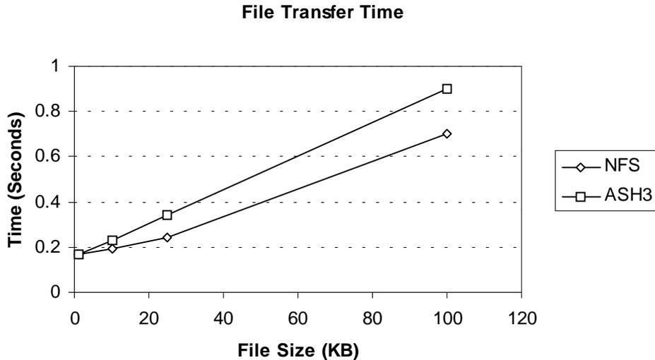
**Figure 5:** Average transfer latency for a remote read operation. Measured 1000 times and standardized for the average latency encountered.
