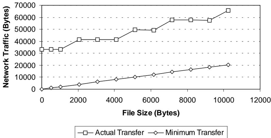
**Figure 6:** Network traffic overhead for a remote copy command versus the amount of data copied.
