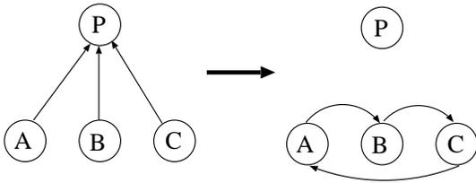
Fig. 2. Simultaneous switching creates loop
