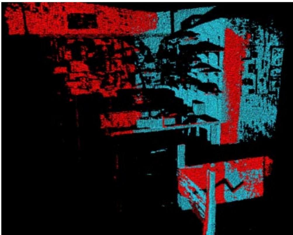
Figure 9: (Top) Registration of view 1 (blue) and view 2 (red) with 41.3% overlap. (Bottom) Registration of view 2 (red) and view 3 (blue) with 20.3% overlap.
