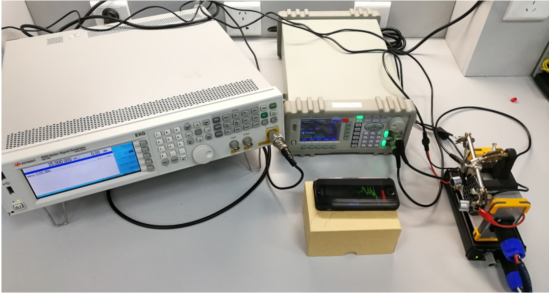
Figure 20: Our benchtop equipment to carry about the proof of concept reproduction of tones heard in Cuba. Note, we would expect emitters to be smaller than a paperback book in practice, if not smaller. We use large equipment because of our general-purpose laboratory.
