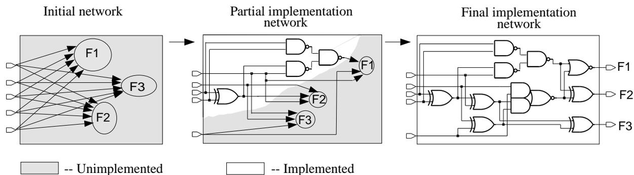
Fig. 2. Illustration of the constructive technology-dependent synthesis
