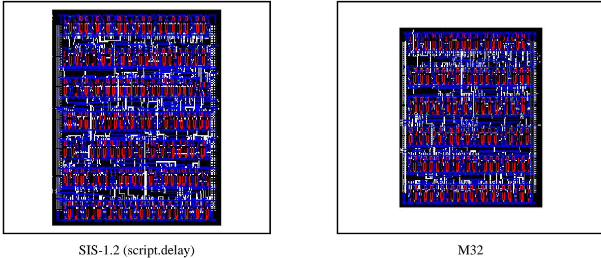
Fig. 6. Cordic relative layout areas (shown to the same scale)
