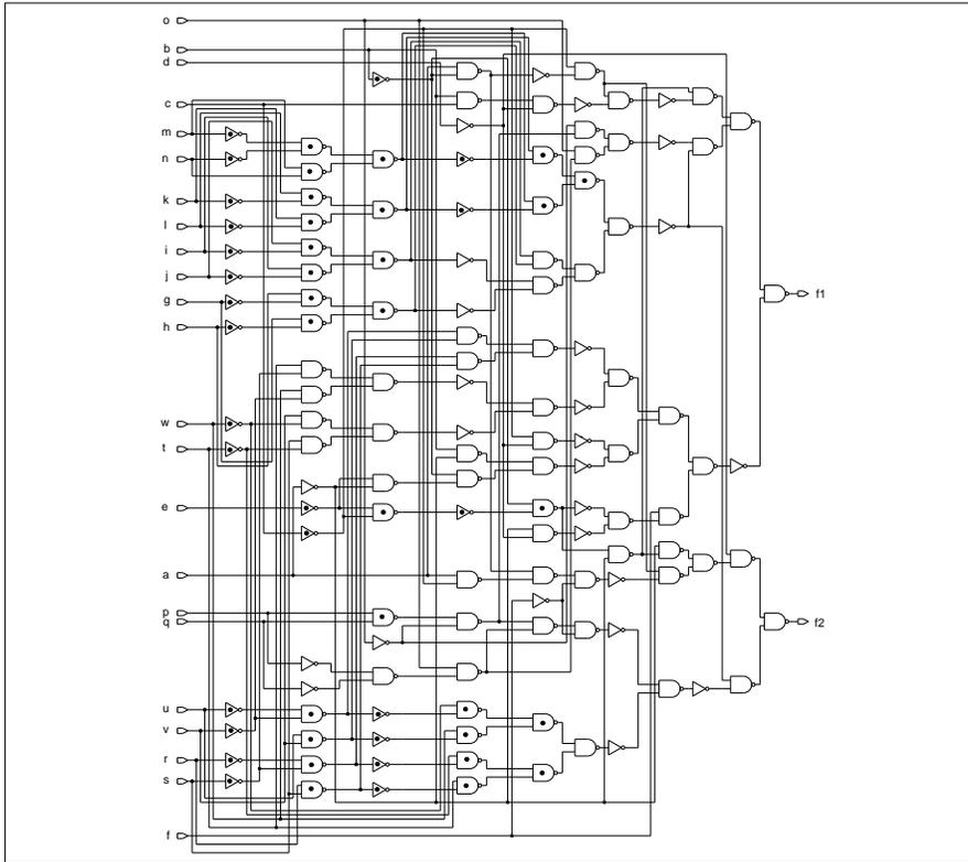
a) Synthesis with topological constraints: 133 gates, 11 levels
