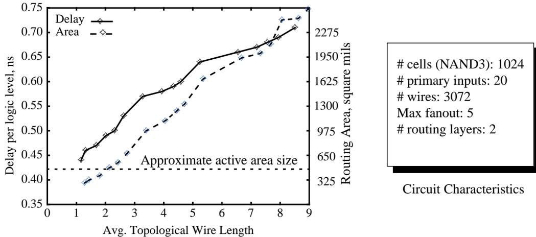
Fig. 1. Effects of wiring on circuit area and delay.
