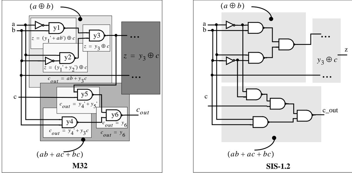
Fig. 5. Synthesis of the full adder in M32 and SIS-1.2
