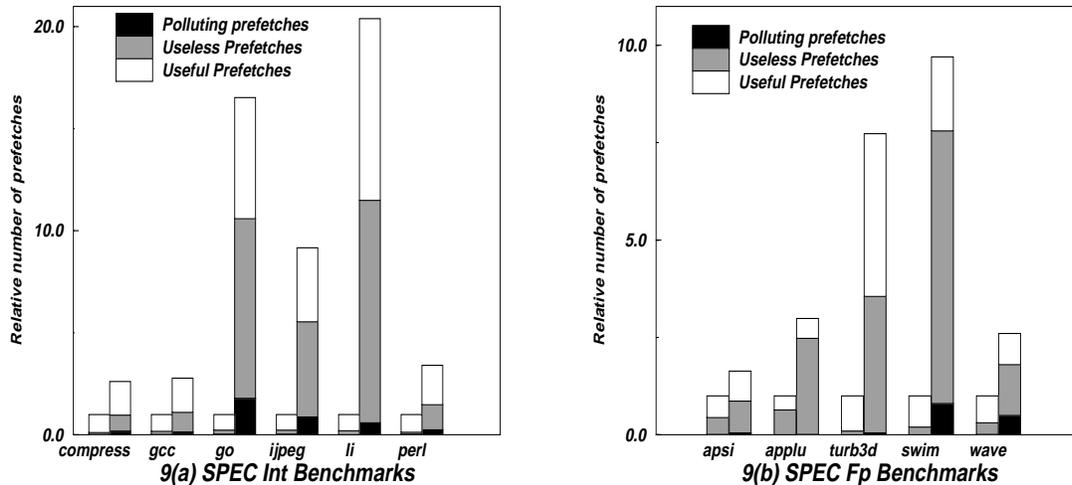
Figure 9: Prefetch Traffic Analysis:Cache: 16KB, 4-way, 32B blocks (left bar = SF-SDP (normalized to 1), right bar = SDP)
