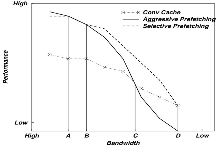
Figure 1: System performance vs Memory bus bandwidth
