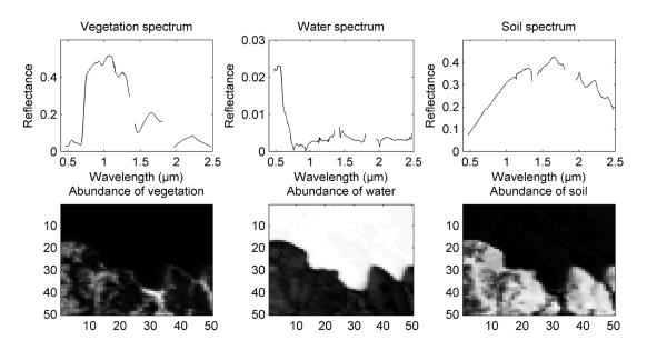
Fig. 8. Top: the R = 3 endmember spectra estimated by the algorithm in the Moffett Field scene. Bottom: the corresponding abundance maps (black (respectively, white) means absence (respectively, presence) of the material).
