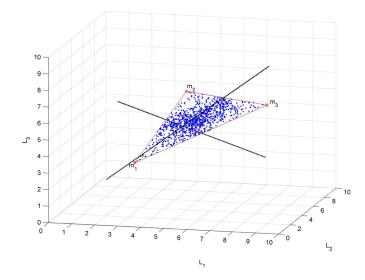
Fig. 2. Example of hyperspectral data observed in 3 spectral bands. The mixed pixels (blue points) belong to the *R*-dimensional convex polytope  $S_M$  (red lines) whose vertices are the endmembers spectra  $m_1, \ldots, m_R$  (red stars). The first two principal axes estimated by a PCA appear in dashed lines and define the projection subset  $V_K$ .
