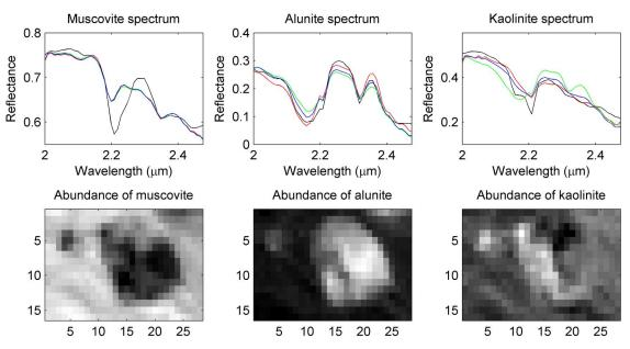
Fig. 10. Top: the R = 3 endmember spectra estimated by the Bayesian (red lines), N-FINDR (blue lines) and VCA (green lines) algorithms in the Cuprite scene, compared with the signatures extracted from the USGS spectral library (black lines). Bottom: the corresponding abundance maps estimated by the Bayesian algorithm (black (respectively, white) means absence (respectively, presence) of the material).
